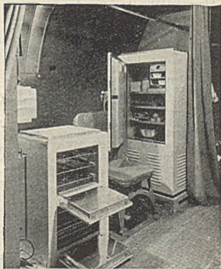
G.E.C. equipment in a Dutch liner includes a lightweight refrigerator (right) with capacity of 3.23 cu. ft. and thermostatic control. The hot cupboard has heating elements in the bottom and back of each compartment, the maximum loading being 750 W
