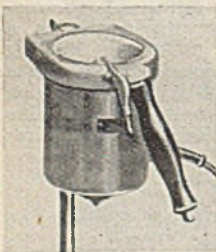
Barlow-Whitney one pint electric wax dropper
