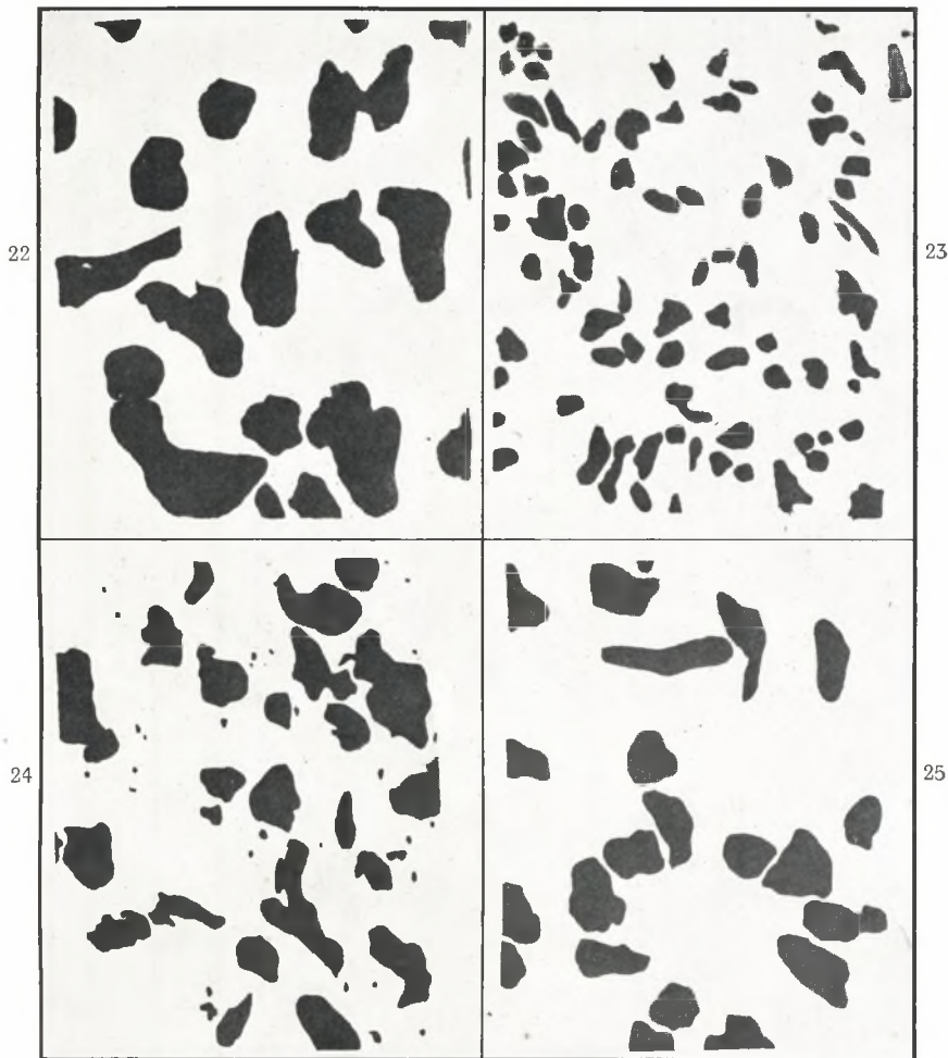
FIG. 22.—Aluminium Powder, 60/72 Mesh. \times 27 .
