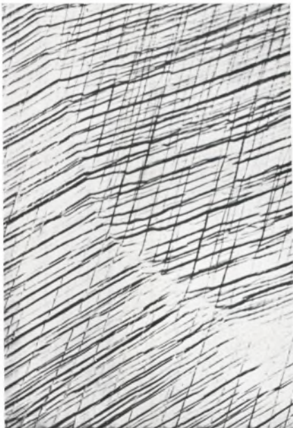
FIG. 11.—Influence of Grain Boundary on the Slip-Deformation of Two Adjacent Boundaries. \times 750 ; reduced 25% in reproduction.
