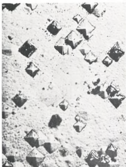
FIG. 2.—Octahedral Etch-Figures on a Single Crystal of Copper Having Its Surface Parallel to a (100) Face. \times 500 ; reduced 25% in reproduction.
