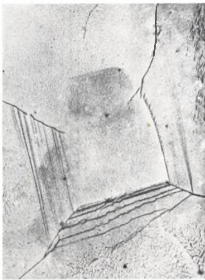
FIG. 27.—Successive Displacement of the Grain Boundaries by Recrystallization During the Course of One and the Same Heating at 600^{\circ}\text{C} . \times 600 ; reduced 25% in reproduction.
