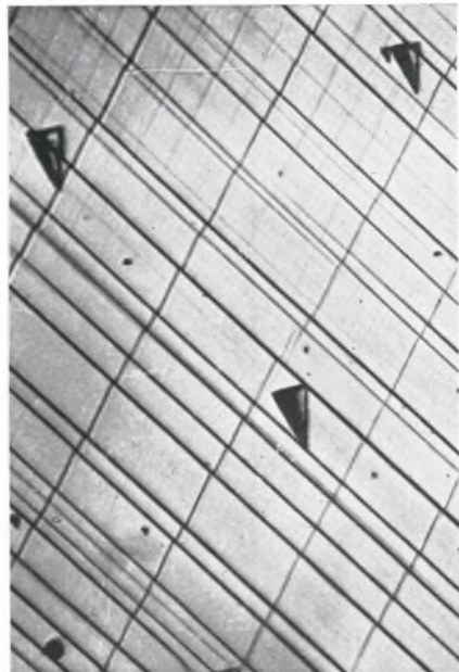
FIG. 10.—Appearance of a Complex Slip on Two Successive Octahedral Planes; Systematic Displacement of the Slip Lines at the Meeting Point with the First System. \times 750 ; reduced 25% in reproduction.
