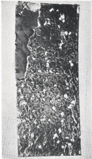
FIG. 9.—Pitting Corrosion on a Sheet Having an Oriented Recrystallization Texture. \times 2 ; reduced 25% in reproduction.
