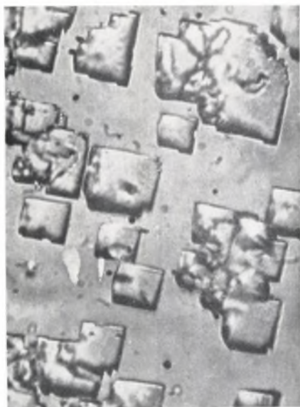
FIG. 4.—Etch-Figures on Aluminium by Electrolytic Polishing. \times 1750 ; reduced 25% in reproduction.
