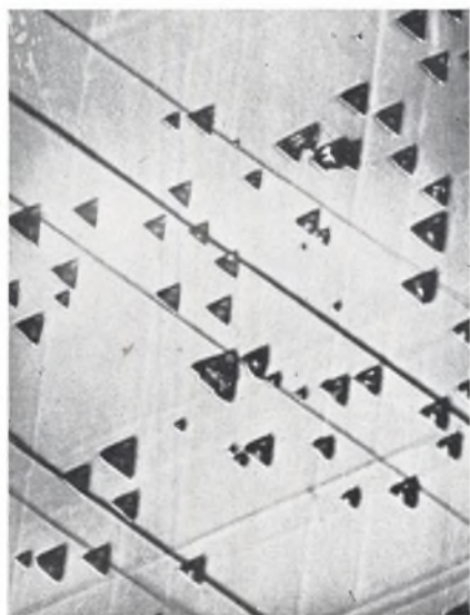
FIG. 16.—Parallelism of the Three Slip Lines with the Sides of the Equilateral Etch-Figures Obtained on a Crystal Surface Parallel to a (111) Plane. \times 650 ; reduced 25% in reproduction.
