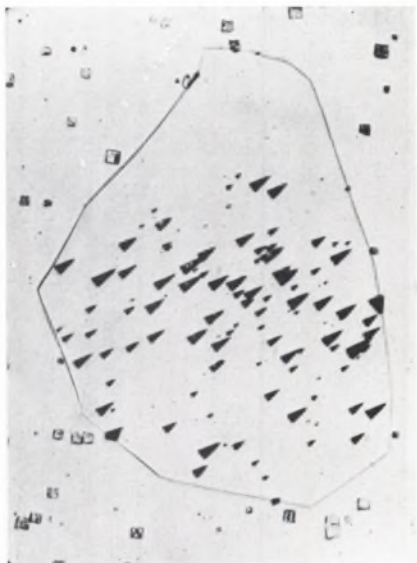
FIG. 5.—The Influence of the Relative Orientation of the Crystals on the Appearance of Their Intergranular Boundaries. \times 500 ; reduced 25% in reproduction.
