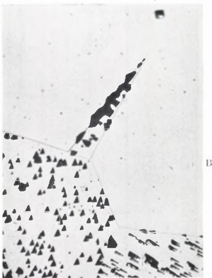
FIG. 7.—Resistance to Chemical Attack of Two Grains Having a Surface Parallel to the (100) Cube Faces. \times 500 ; reduced 25% in reproduction.
