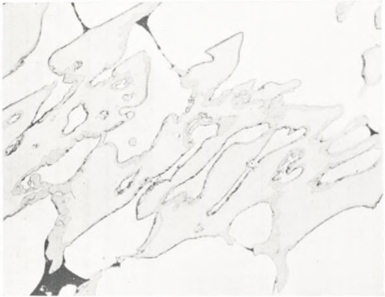
FIG. 3.— MnAl_6 Partly Surrounded by \alpha(Cu-Mn) in Slowly Cooled Alloy Containing Copper 8.0 and Manganese 3.0%. (No MnAl_4 present, due to undercooling.) Specimen etched 1\frac{1}{2} min. in 20% HNO_3 at 70^\circ C. \times 150 .
