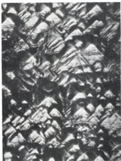
FIG. 3.—Octahedral Etch-Figures on the Same Crystal of Copper Obtained by Electrolytic Polishing. \times 750 ; reduced 25% in reproduction.
