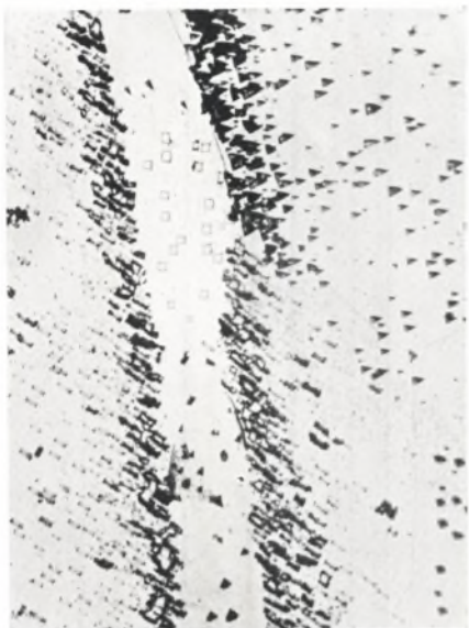
FIG. 1.—Influence of Local Cold Working on the Distribution of Etch-Figures on Refined Aluminium. \times 100 ; reduced 25% in reproduction.
