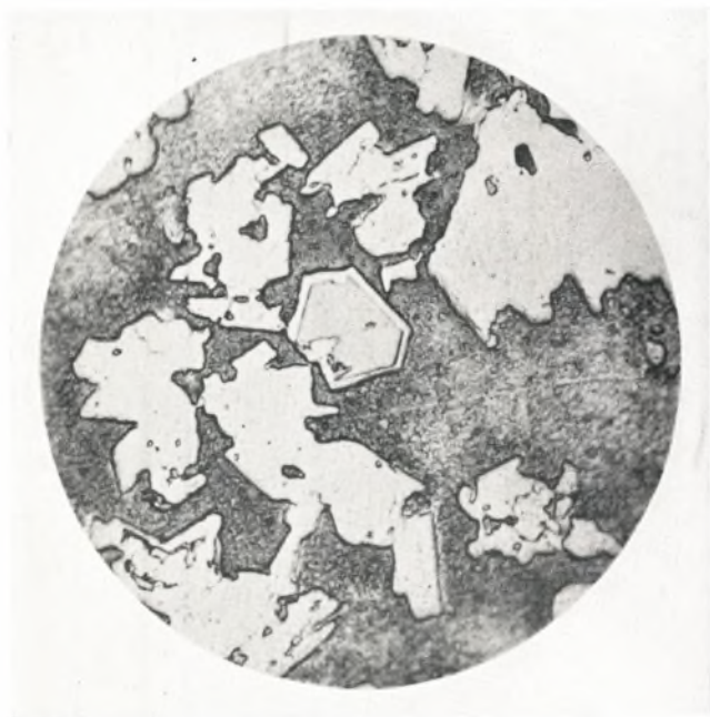
FIG. 1.—Microstructure of an Alloy Containing 7.65% Chromium and 10.22% Zinc After Annealing for 26 Days at 460° C. \times 1000.
