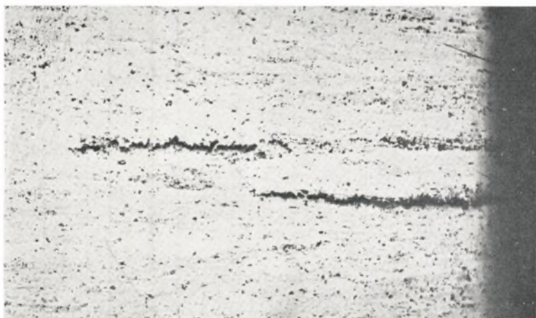
FIG. 5.—Transverse Section at Periphery of 2-Hole Bar in Radial Flow Position. Cracks and radial segregates. \times 50 .
