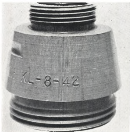
FIGS. 1 and 2.—Components Showing Fan-Shaped Streaks, Parallel on Machined Flat. \times 1\frac{1}{2} .
