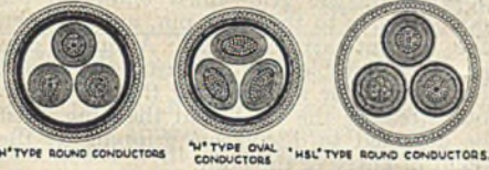
Examples of some solid type paper insulated screened cables
