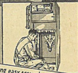
Panel wiring accessible—swinging panel
