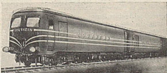
An illustration of the Southern Railway's new double-unit 3 200 H.P. Diesel-electric locomotive to be introduced on main line services to the West of England
