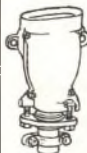
Flat type box for twin, 3-core and 4-core P.I.L.C. and armoured cables.
