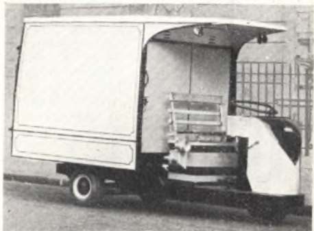
A "Brush-Bred" "Pony" truck, one of five Brush battery-electric vehicles seen at the Dairy Show, Olympia
