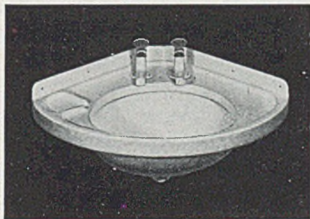
Fig. 3.—Aluminium wash-basin as used on air liners prior to the outbreak of war.
