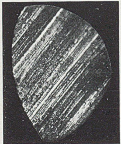
Fig. 15.—Sintered carbide tool edge not diamond lapped. (Equivalent magnification in reproduction 80 diameters.)
