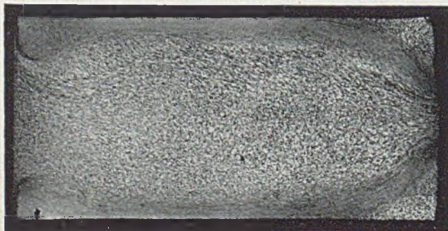
Fig. 3 (Above).—Section of billet with macro etched surface illuminated by diffused light. Compare with Fig. 7, opposite. (Equivalent magnification in reproduction = \frac{1}{4} linear.)
