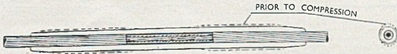
Fig. 5.—Connector for steel-cored aluminium conductors. This diagram shows form before and after attachment has been effected by compression.
