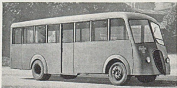
Fig. 1.—Prefabricated light-alloy body for the Shanghai Tramway Co. Twenty vehicles are now in service.
