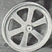
SMALL SHEAVE - Gravity die-castings by Dialoy Ltd for child's all-weather sledge and sleigh for Metal Products Ltd, Belfast
