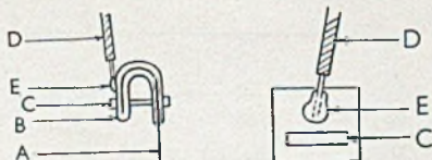
Fig. 128 (left).—Side view of termination of electrode foils. Fig. 129 (right).—End view of termination of electrode foils: A, aluminium foil tab; B, tinned copper strip; C, tinned steel clip; D, braided flexible wire; E, soldered joint.
