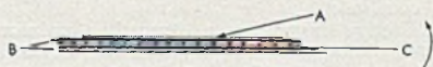
Fig. 130.—Showing arrangement of layers: A, anode; B, cambrics or paper; C, cathode. Arrow shows direction of winding or rolling.
