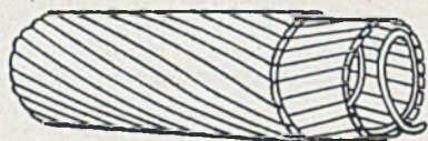
Fig. 5 (above).—Variation in design of hollow conductor. In the production of this type, electrically suitable aluminium alloys can be substituted for copper.
