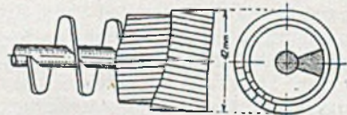
Fig. 4 (below).—Method of construction of tubular conductor in aluminium. This system is usually employed in the manufacture of steel-reinforced aluminium cables of this type for high-voltage overhead lines.
