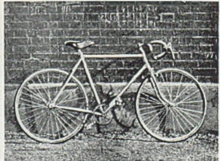
Fig. 23.—Caminargent all-light-metal bicycle; road-racing model weighing 17 lb.
