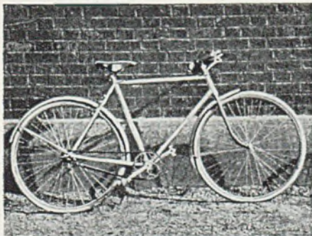
Fig. 22.—The Caminargent all-light-metal bicycle; Roadster model.
