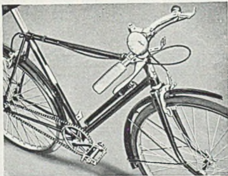
Fig. 26.—Bicycle by J. A. Phillips and Co., Ltd. The frame in this instance is of steel, but mudguards, pedals, hubs, front and rear cable brakes (calipers and levers), adjustable stem, handlebar bend and wing nuts are all in light alloy.
