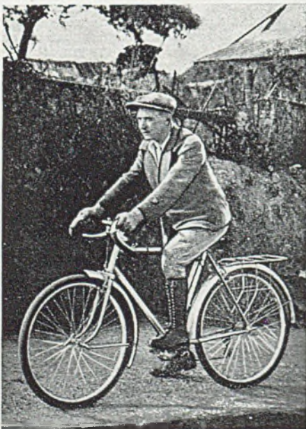
Fig. 19.—A Caminargent bicycle. The touring model shown here weighs, when fully equipped, 22.9 lb.
