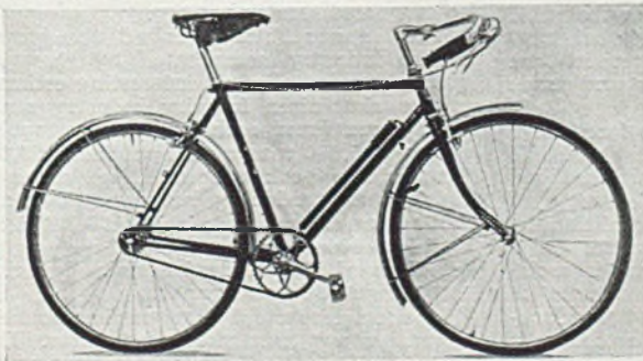
Fig. 27.—In this later model of the Phillips bicycle, which was exhibited at the Exhibition "Aluminium—From War to Peace" at Selfridges, not only are the components listed in Fig. 26 (above) in light alloy, but, in addition, the chain wheel is also in light metal.
