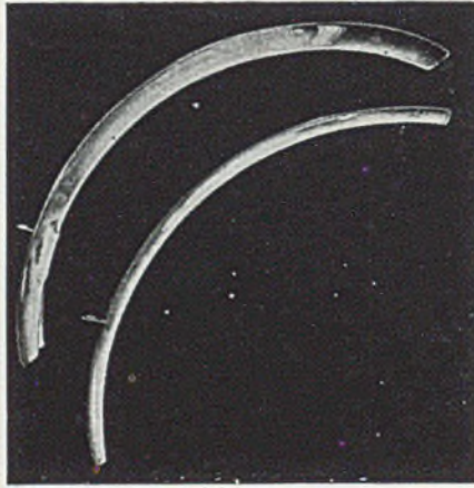
Fig. 7.—Illustrated here is a set of duralumin mudguards.
