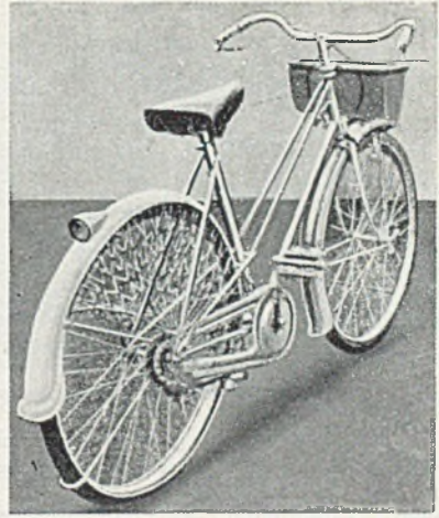
Fig. 16.—The "Superleggera" model bicycle of the Italian "Gloria" concern. Note in particular the double frame construction. This assembly weighs about 8 kilos.
