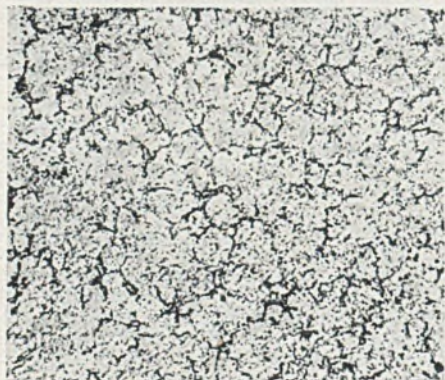
Fig. 31.—Microstructure Type 218 metal, centre of bar; gauge length C' test bar (equivalent magnification in reproduction = 300 diams.).
