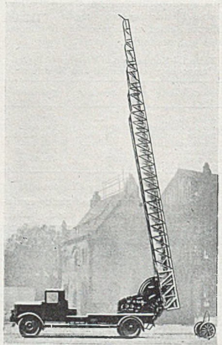
ILLUSTRATED above and at the left is the light-alloy fire escape of the Brussels Fire Brigade, shown in the elevated and fully extended positions respectively. The height of the escape, in the latter case, is 42 metres.
