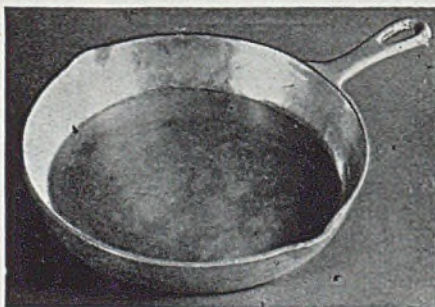
Fig. 1.—Frying pan for contact heating cast in pure magnesium. This has been in continual use since July, 1945, over an open gas flame; no distortion of the bottom has occurred. After use it has been regularly cleaned with steel wool and soap flakes together with washing soda; it still remains bright and shows no sign of corrosion although, after standing idle for a few days, it does acquire an easily removable not-unpleasant-looking whitish film (Courtesy Dominion Magnesium Co. Ltd.)
