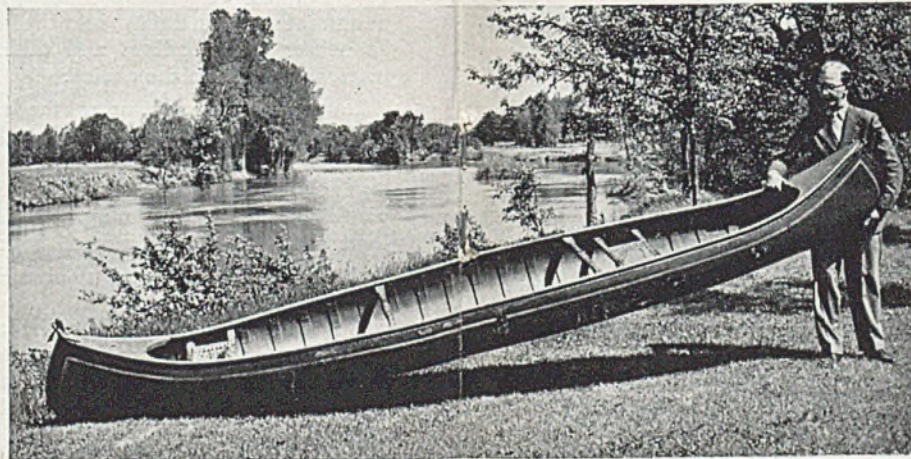
Fig. 1 (above).—Shown here is a magnesium-alloy canoe after ten years' service. It should be noted that, in spite of the fact that the alloy used in this case was not of high purity, and despite the fact that the canoe was not repainted during this period, no corrosion has occurred. Fig. 2 (below).—View of part of the exposure station at Wilmington, N.C.
