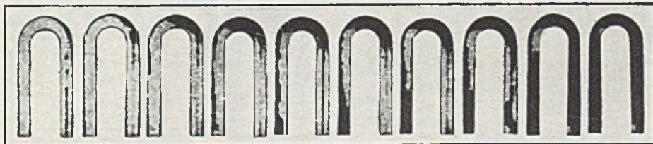
Fig. 5.—Progress of filling for a rounded U-type mould. Reading from left to right, the illustration at the extreme left shows the mould 6 \times 10^{-3} secs. after pouring has commenced. Succeeding illustrations show the mould at intervals of 8.5 \times 10^{-3} , 17 \times 10^{-3} , 24 \times 10^{-3} , 34 \times 10^{-3} , 38 \times 10^{-3} , 54 \times 10^{-3} , 58 \times 10^{-3} , 72 \times 10^{-3} and 86 \times 10^{-3} secs., the last illustration showing the mould completely filled.
