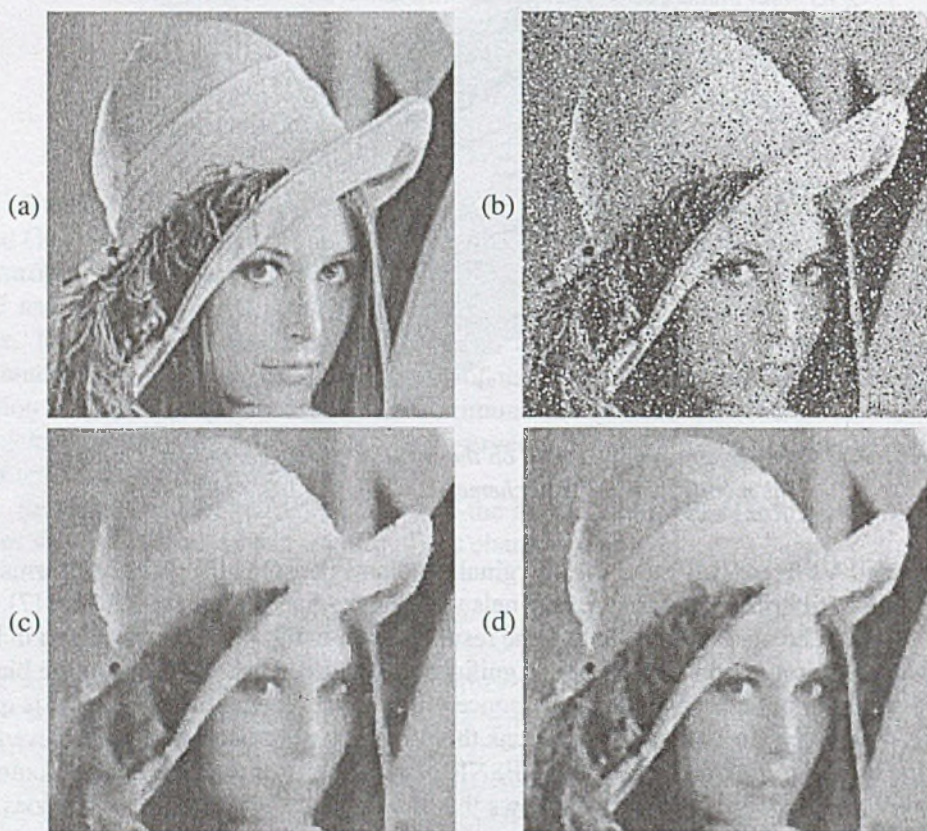
Fig. 8. Comparison of the efficiency of the standard AD with the new method: (a) LENA image, (b) noisy image: Gaussian ( \sigma = 30 ) and impulse noise ( p = 0.3 ), (c) optimal output of AD, (d) best output of the modified BAD with VMF prefiltering
