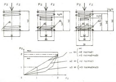
Fig.5. Construction variant and the possible changes in the Pz loading of an assembly in relation to the deflection fz
