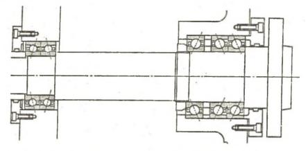
Fig. 1 Bearing Arrangement of the Spindle Housing
