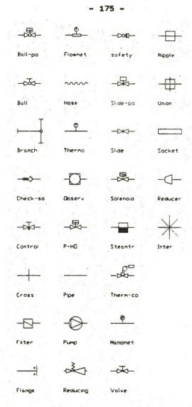
Fig. 1. Set of schematic symbols for pipelirie elements
