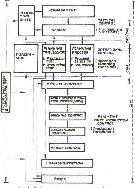
Fig. 1 Reference Model of Manufacturing Control System
