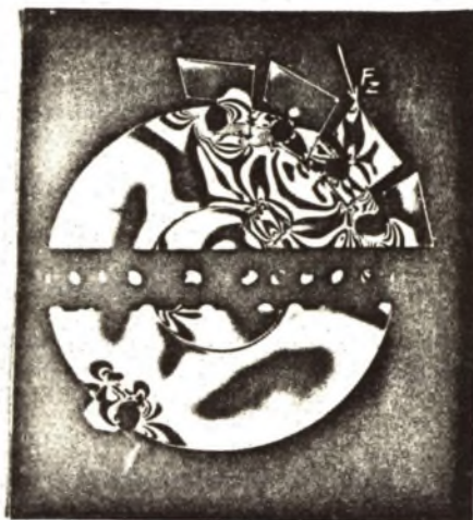
Fig.3. Stress distribution in basic body of tool, fixing pressure 20 MPa + cutting force F_z
