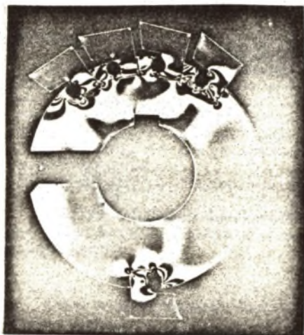
Fig.2. Stress distribution in basic body of tool, fixing pressure 10 MPa
