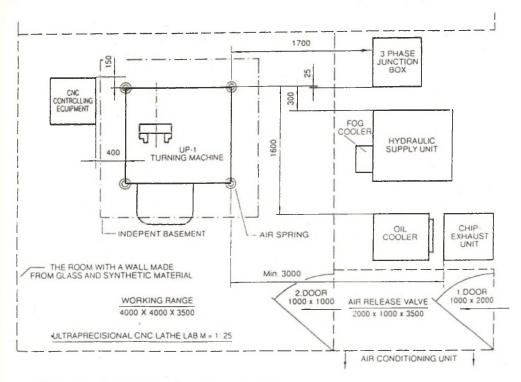
Fig. 1, Ground-plan of the ultraprecision lathe laboratory
