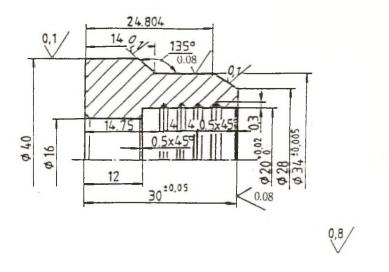
Fig.3. Part made of hardened steel
