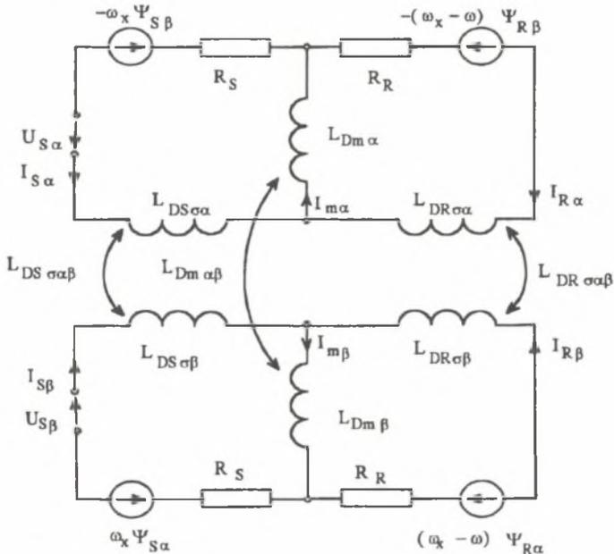
Fig. 1. Equivalent circuit of the asynchronous motor considering the effect of magnetic saturation of the motor
