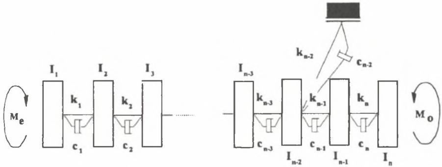
Fig. 2. Dynamical model of the driving system
