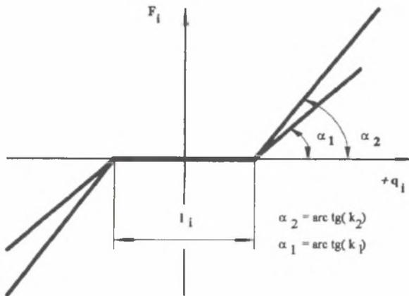
Fig 4. Course of the function simulating clearance and varying stiffness for the spur gear
