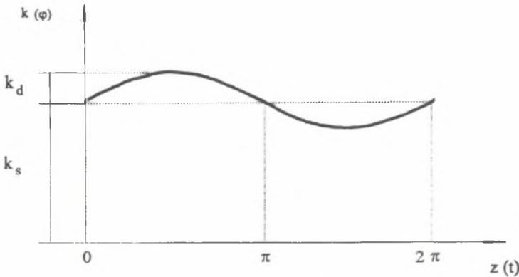
Fig.5. Varying stiffness of spur gear meshing simulated by harmonic function
