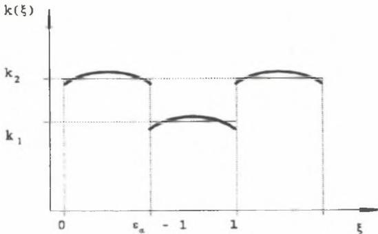
Fig 3. Varying stiffness of meshing in spur gear
