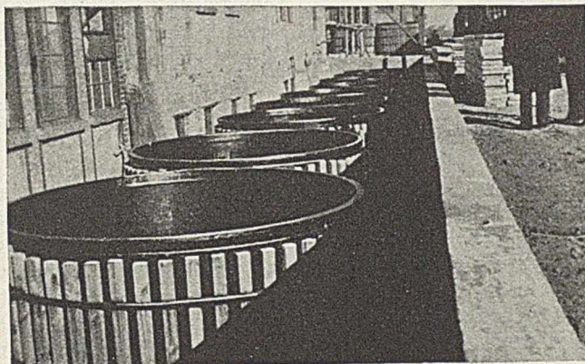
Tanks of synthetic resin-asbestos reinforced by wooden staves
