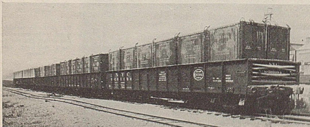
Fig. 3. Transporting pebble lime in 200-cu.ft. containers with drop-bottom outlets
