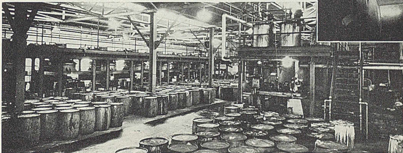
Nitrocellulose dope is made in mixers at left. Pigment is dispersed in castor oil with the colloid mill (right)
