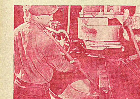
4 The salt is drawn from the open pan to a centrifuge from which it passes to a Monel lined rotary dryer
