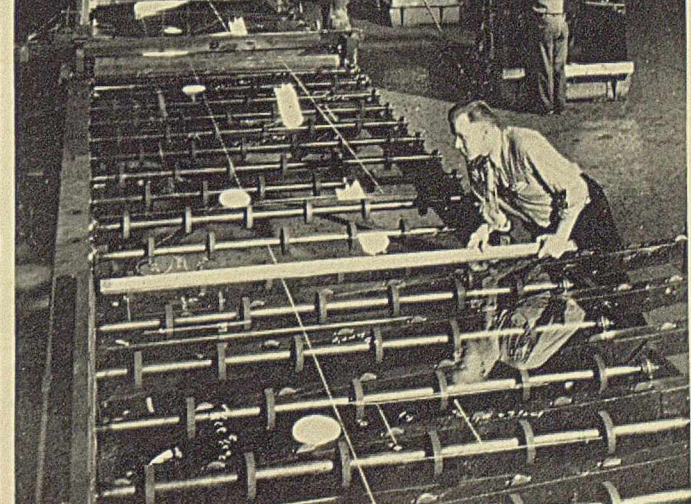
12 Marked sheets or plates pass along the line to the cutting machine where they are cut into the sizes required by the customer
