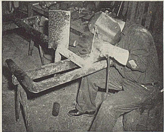
This rotor agitator was fabricated from 2½-in. steel pipe and ¾-in. plate for the paddle. It was built in the shop of the Amino Products Co., which is equipped with a 150-amp. arc welder
