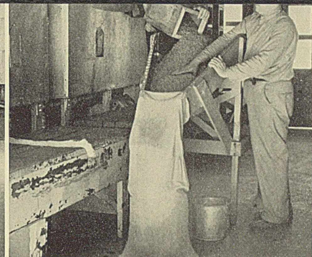
9 Powder is put into covered cars which are sent to the solvent recovery building
