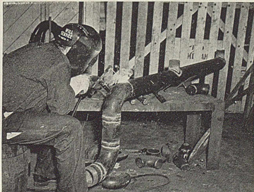
This rotor agitator was fabricated from 2½-in. steel pipe and ¾-in. plate for the paddle. It was built in the shop of the Amino Products Co., which is equipped with a 150-amp. arc welder
