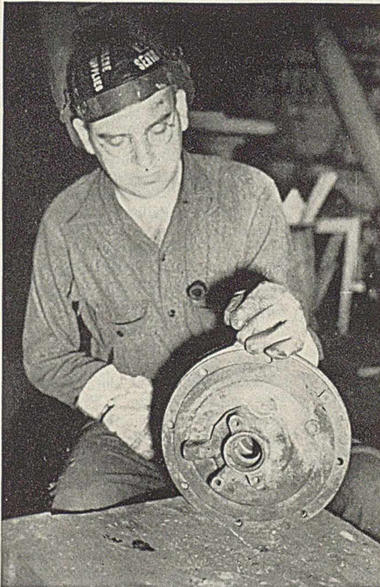
This 5-minute arc welding job saved $42.50. The pitted pump housing would have cost $44 for replacement. "Aerisweld" electrodes were used
