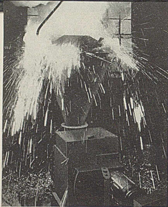
Thermit reaction in welding heavy crankshaft
