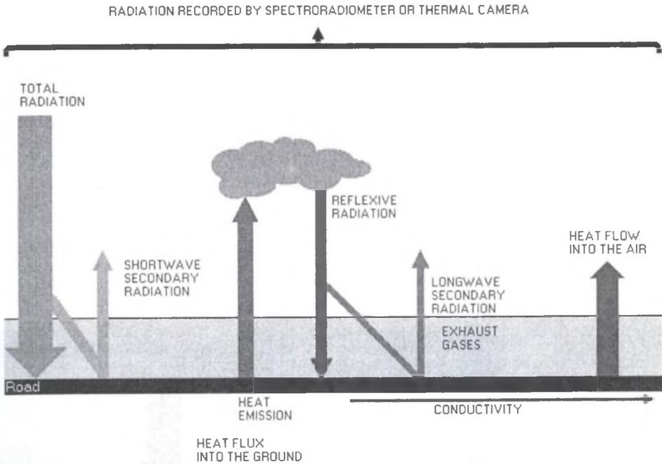
Fig. 1. Qualitative representation of heat streams at the road surface
