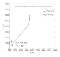
Fig.3. Trajectories of ships in an encounter situation in an open area; simulation time 1200 [s]; positions (x) at 300 [s] time intervals;
