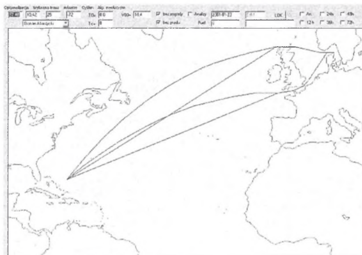
Fig. 1. Great circles and rhumb lines for various routes of a ship running through the English Channel and Pentland Strait
