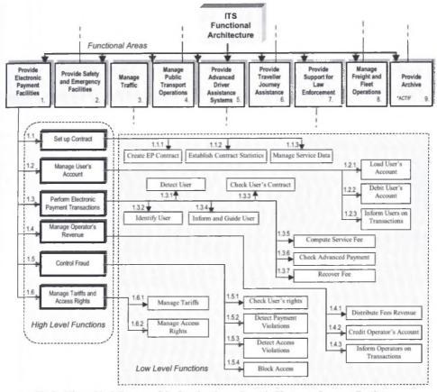
Fig.2. Hierarchical diagram of the functional area Provide Electronic Payment Facilities
