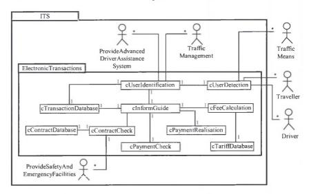
Fig.6. Class Diagram (classes drawn in a simplified view)
