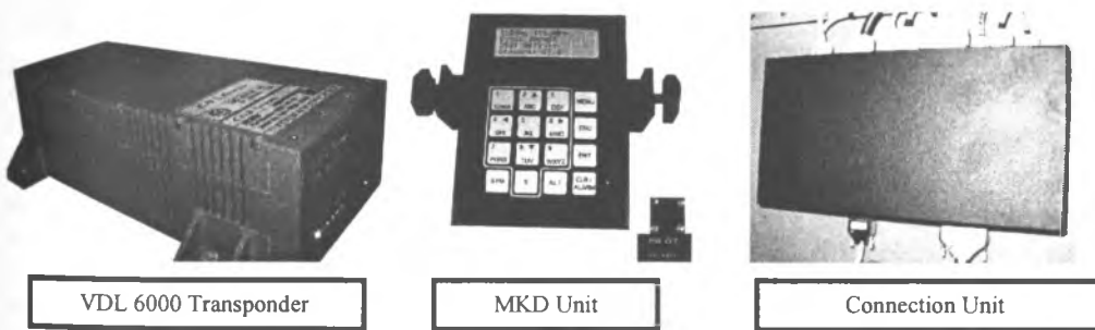
Fig.2. MKD Unit, Connection Unit and VDL 6000 Transponder in the CNS VDL 6000 AIS system
