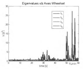
Fig.7. Rolling quality of an ICE wheel set, running on a bad conditioned track section
