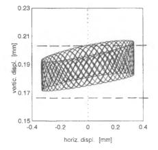
Fig.3. Simulation of the axle bearing orbits of an ICE wheel set, which undertakes bending/torsion vibrations due to static and dynamic out-of-balance (SZOLC 1995)
