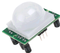
Figure 190: PIR motion sensor HC-SR501 109)
