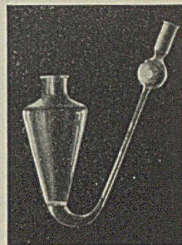
FIGURE 18. YEAST AERATION VESSEL AFTER KLUWYER
