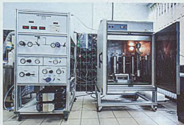
Core flooding system
