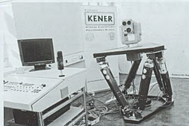
Fig. 2. Test stand for the shipboard motion simulator for investigating the sea motion compensation system of the observation turret.
