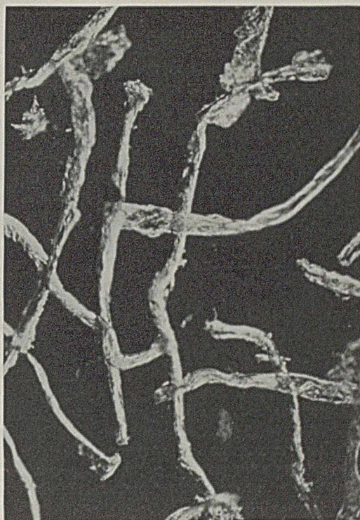
FIGURE 3. PHOTOMICROGRAPH OF RUN 4 Light tackle, 3 per cent consistency, 150 X
