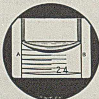
Field of view on burette with all-round graduations, with eye in correct position, i.e. no parallax on critical line A—B
