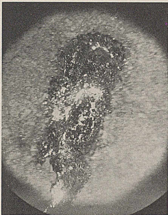
FIGURE 5. IRIDIUM-SILVER, 1 TO 7 Magnification, \times 20 . Weight, 30 mg.
